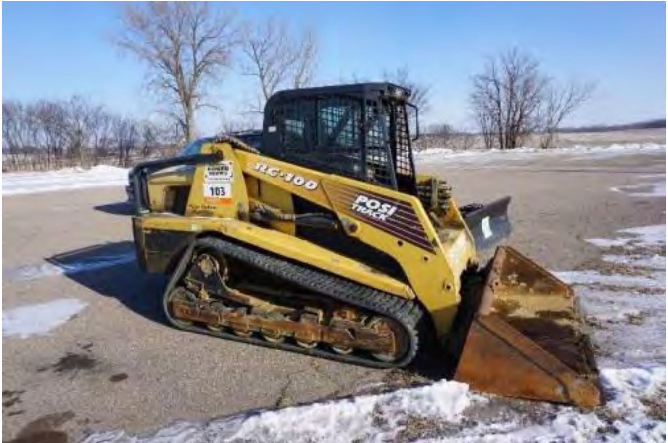
The ASV Skid Steer with plow is a specialized low PSI vehicle for plowing the Engineered Material Arresting System (EMAS) - Airport Vehicle #38
