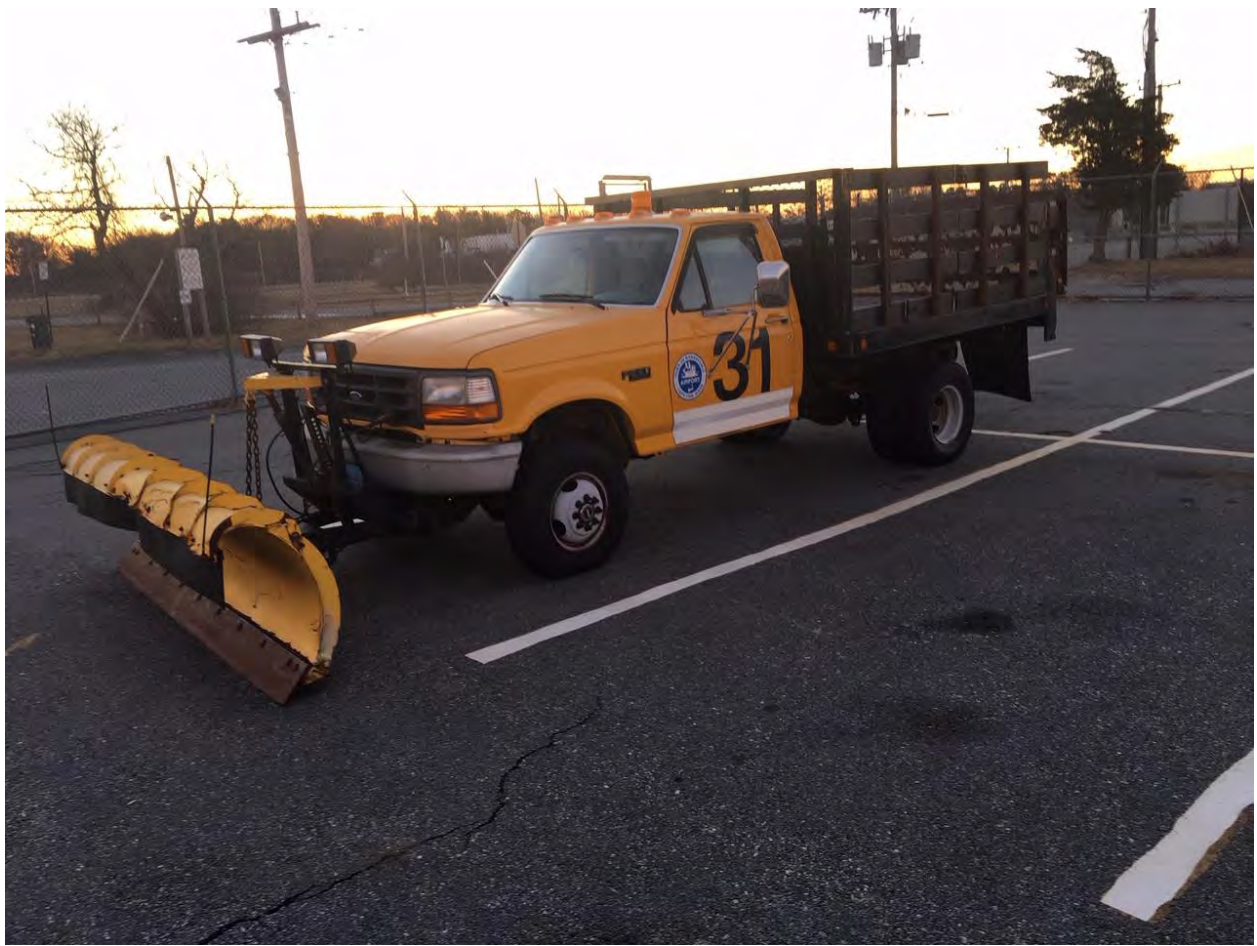
Snow Removal Equipment (SRE) (Ford F350 – Heavy Duty Vehicle with Plow and lift gate)
